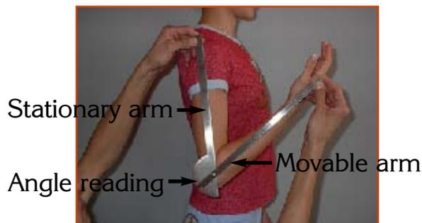
*Figure 1 Parts of a Goniometer*
